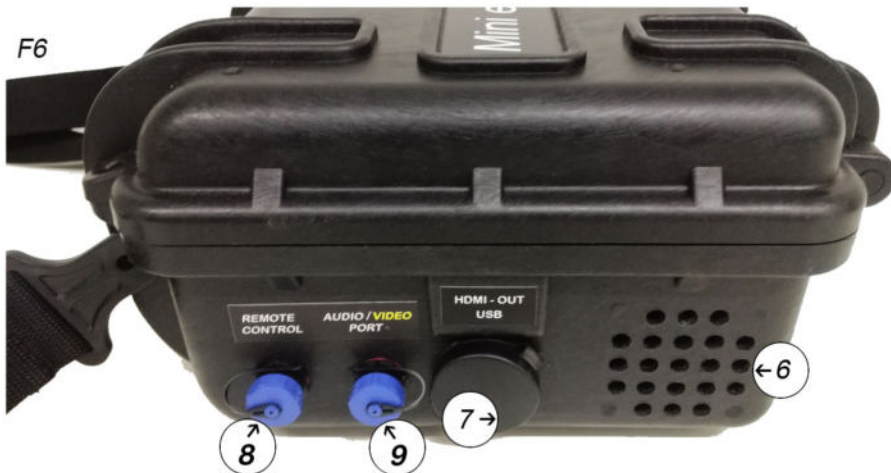
Figure 5 - Audio/Video umbilical sockets
