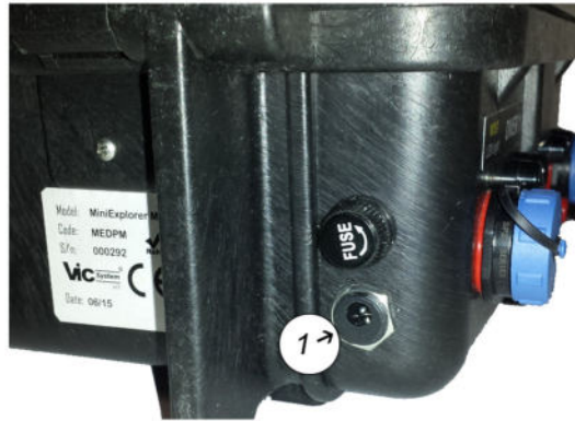
Figure 7 - Plug for charging and power supply
